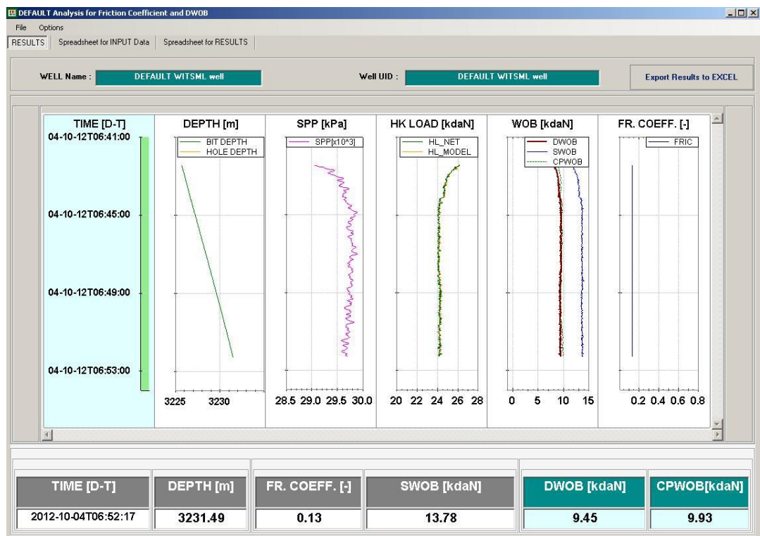
FIGURE 6 TIME BASED ANALYSIS TO ESTIMATE FRICTION COEFFICIENT AND DOWNHOLE WOB
