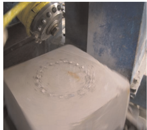
Fig. 5. Single-row insert work piece used to run the indentation test (Hareland et al., 2010).
