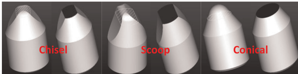
Fig. 8. Cross section area of the common cutter types as a function of height of cutters (Hareland et al., 2011).
